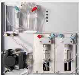
Sample Introduction by sequential injection and continuous flow
