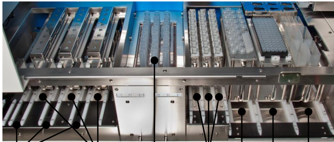
4 Sample tip holder 3 Cartridge/Waste tube holder 5 Lysate unit Sample holder slot 2 Reagent tip holder 1 Reagent container holder slot Reagent container holder slot
